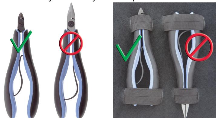
New Biospring® (1) compared to a deformed spring (2) which was removed from a pair of pliers that was stored with the handles forced closed and the spring still engaged at both ends.
