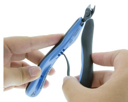
5. Using the adjustment port closest to the joint will provide a lighter tension and the position furthest from the joint provides the greatest tension.
