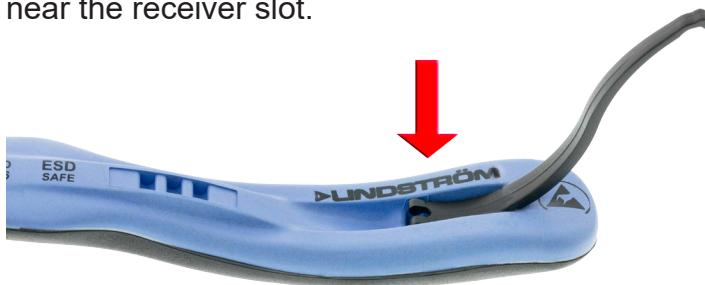
2. Simultaneously push the wide end of spring into receiver slot (arrow 1) and rotate thin knob end up (arrow 2).
